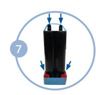
If tape is applied to column assembly, remove tape. To install new columns, first remove the four (4) dust caps from the new columns. Make sure there is no dust or debris where the dust caps were located.
