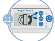
Press and hold the plus (+) and (-) minus button for 5 seconds. The screen will display the 'sieve reset' informational icon. Release the buttons once the 'sieve reset' icon is displayed on screen.
