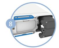
Insert the new columns into the device immediately after removing the dust caps. DO NOT leave the column ends exposed. Push the columns into the device as far as possible.
