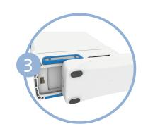
Remove the battery from the device.
