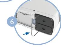
While holding the button open, slide the column assembly out of the device by pulling on the column pull handle.
