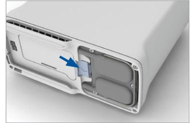
6. While holding the button open, slide the column assembly out of the device by pulling on the column pull handle.
