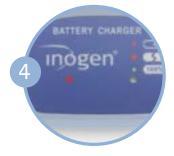
When the battery is in the correct position, a solid red light will indicate that the battery is charging.
